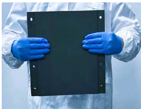
Fig. S1 Macrophotograph of the coated C/CA panel with a size of 300 mm×300 mm×25 mm
