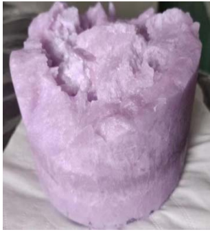
图 2 熔融法制备的多晶原料 Fig. 2 Polycrystalline material prepared by melting method
