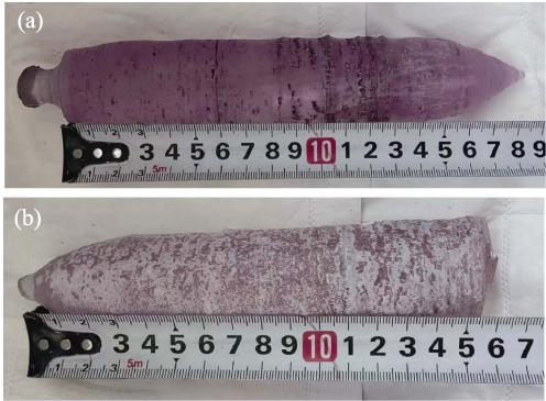
图 3 提拉法生长的 Nd:YLF 晶体 Fig. 3 Nd:YLF crystals grown by Czochralski method (a) Crystal grown with polycrystalline material prepared by melting method; (b) Crystal grown with mixed component raw materials
