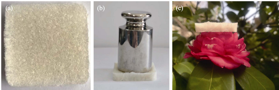
图 4 62.5PMo-LDHs+BA/CNFs 气凝胶的(a)外观形貌及其置于(b)砝码下和(c)花瓣上的照片 Fig. 4 Morphology of 62.5PMo-LDHs+BA/CNFs aerogel (a) and digital photos when it placed (b) under weight and (c) on petals
