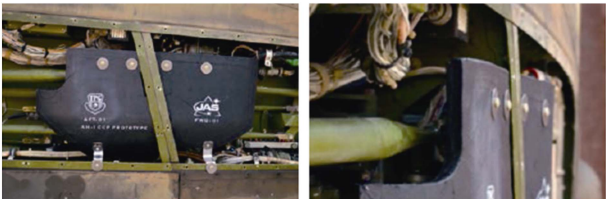
图 4 曲柄外壳带曲率陶瓷装甲安装示意图 [51] Fig. 4 Curved ceramic armors of bell crank housing [51]
