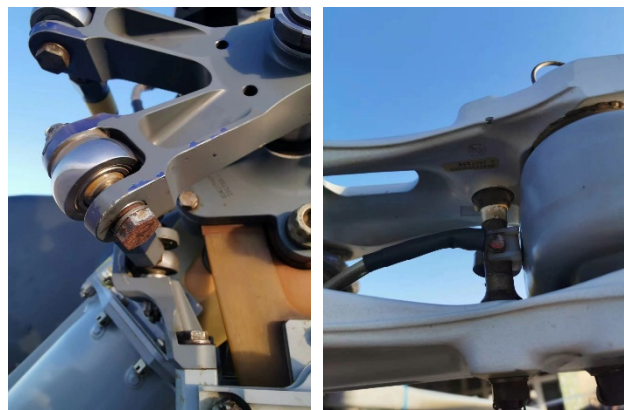
图 3 旋翼连接结构外场腐蚀 [38] Fig. 3 Field corrosion of rotor connection structures [38]
