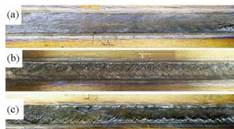
图 1 激光束不同扫描速度下复合涂层的表面宏观形貌 Fig. 1 Macromorphologies of composite coatings under different scanning speed conditions (a) 5.83 mm/s (T1); (b) 6.67 mm/s (T2); (c) 7.50 mm/s (T3)
