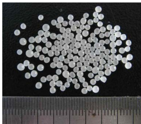
图 2 造孔剂蜡球的形貌 Fig. 2 Appearance of the pore former of wax spheres
