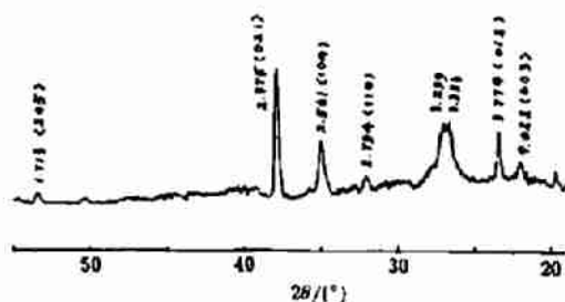
图 6 经 800°C×1h 烧结后的碳化硼 X-ray 衍射图 Fig.6 X-ray diffraction pattern of oxidized boron carbide after 800°C×1h sintered
