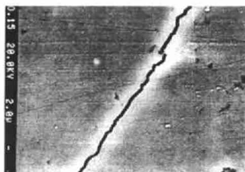
图 4 SiC/SiC w 复相陶瓷裂纹扩展过程的 SEM 照片 Fig. 4 SEM micrograph of crack propagation in SiC/SiC w composites
